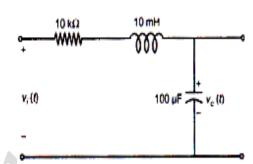
Q5.24. The transfer function  $H(s) = \frac{V_o(s)}{V_i(s)}$  of an R-L-C circuit is given by
