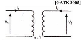
Q3.13. A two-port network is represented by ABCD parameters given by
