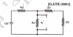
Q1.23. The minimum number of equations required to analyze the circuit shown in figure is [GATE-2003]
