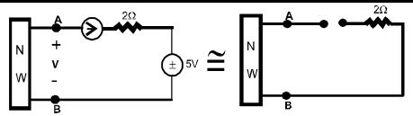
So calculation of  $V_{AB}$  is not possible with network information, so (d) option is correct.
