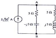
Q5.35. In the circuit shown,  $V_c$  is 0 volts at t = 0 sec. For t > 0, the capacitor current  $i_c(t)$ where t is in seconds, is given by: [GATE-2007]
