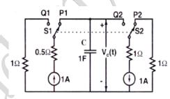
Assume that the capacitor has zero initial charge. Given that u(t) is a unit step function, the voltage  $V_C(t)$  across the capacitor is given by:
