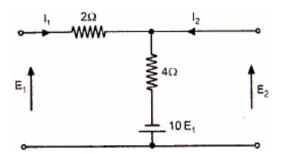
Q3.8. The admittance parameter  $Y_{12}$  in the two-port network in figure is: [GATE-2001]
